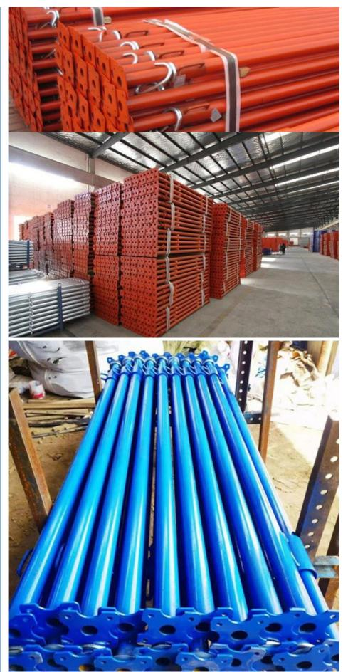
Maintenance and Care: Check for Corrosion and Damage: Regularly inspect support rods, threads, nuts and other components to ensure there is no corrosion, rust or obvious damage. If any problems are found, damaged parts should be repaired or replaced promptly.
